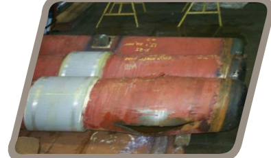
Pipe Body Failure @ 4,260 psi
